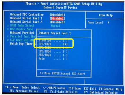
6. Verify that the "Onboard Serial Port 1" option is "3F8/IRQ4".
